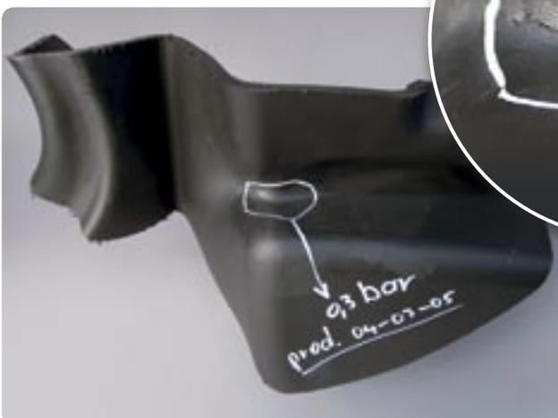
distribution, and in addition it had bad sintering with bubbles in the same area. The tank was undergoing quality inspection by supplying low pressure to check for leakage. The customer changed to a material with higher MFI. This solved the problems related to material distribution and sintering, but new problems occurred. Now the tank broke, due to lower physical properties of the new material.
