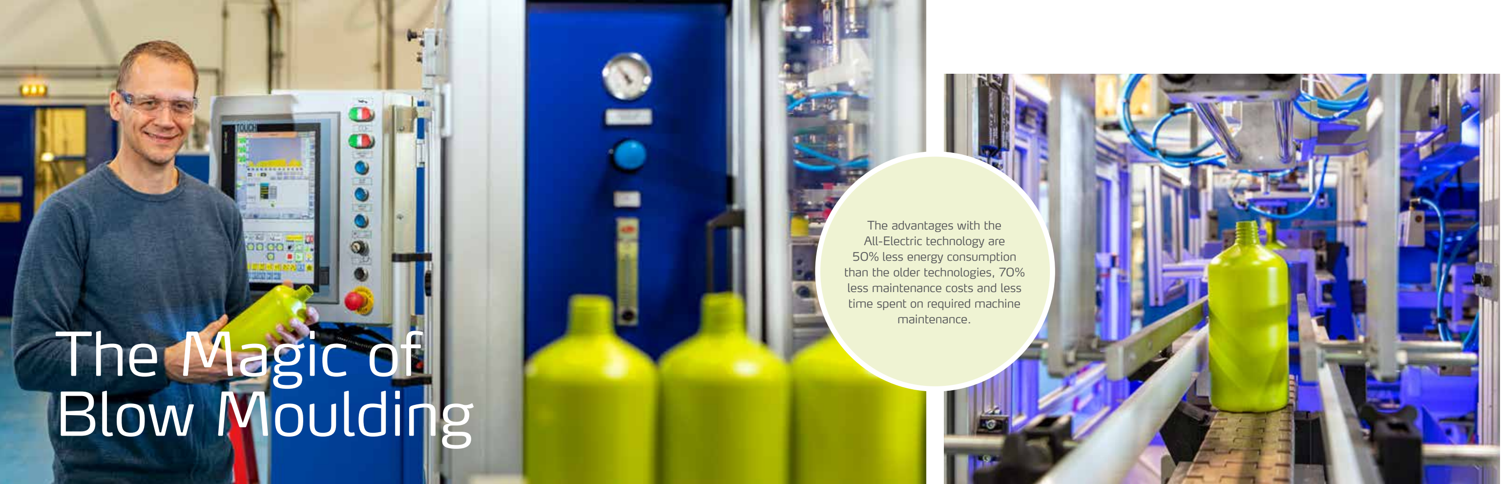
Magic monolayer and CoEx 3-layer machine. Fully electric with 3 extruders with a screw diameter of 38mm and L/D of 24. Different moulds from 0,5 to 3 litres can be used, many moulds are available in the Application Centre. Leakage test of bottles are done in-line on the machine.
