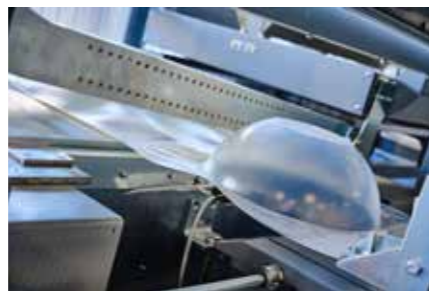
» Thermoforming of sheet.
