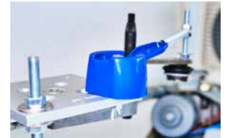
» Hinge testing of a flip top cap.
