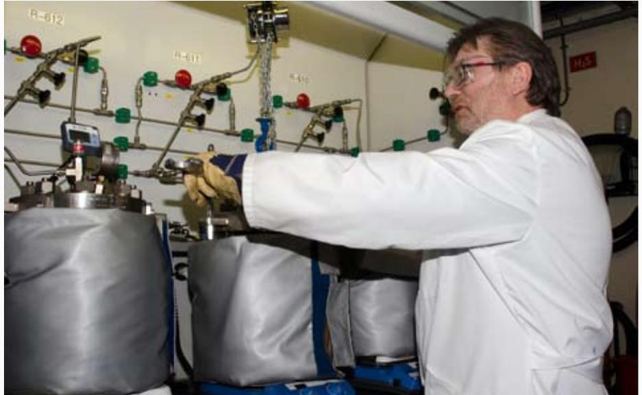
The exposure testing is typically followed by mechanical testing, hardness, swelling, additive residues and microscopy evaluations. Life-time prediction is crucial since materials are expected to have very long life time, also in critical environment. Norner typically uses Arrhenius plot to calculate this.
