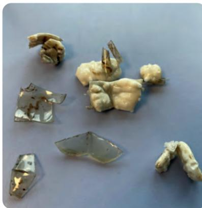
Figure 3 (Left) Popping and (right) lump formation (along with degradation) due to a combination of CO<sub>2</sub> absorption and slow cold crystallization due to the presence of high amounts of 100% recycled PET.
