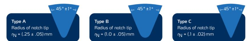
**Figure 2** Bottom radius in Charpy test specimen.
