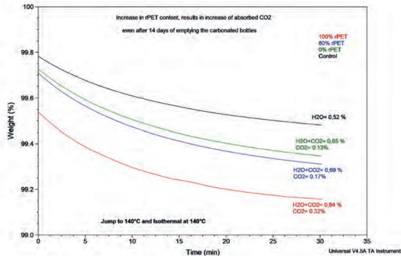
Figure 2 TGA isothermal analysis at 140°C
