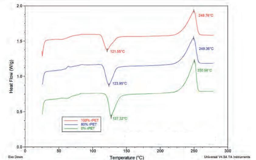
DSC First heating: increasing rPET leads to higher crystallisation temperature.
