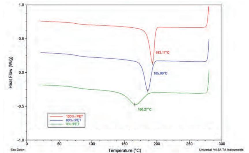
DSC First cooling: increasing rPET leads to higher crystallisation temperature.
