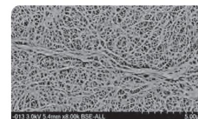
SEM photo of a Battery Separator Film
