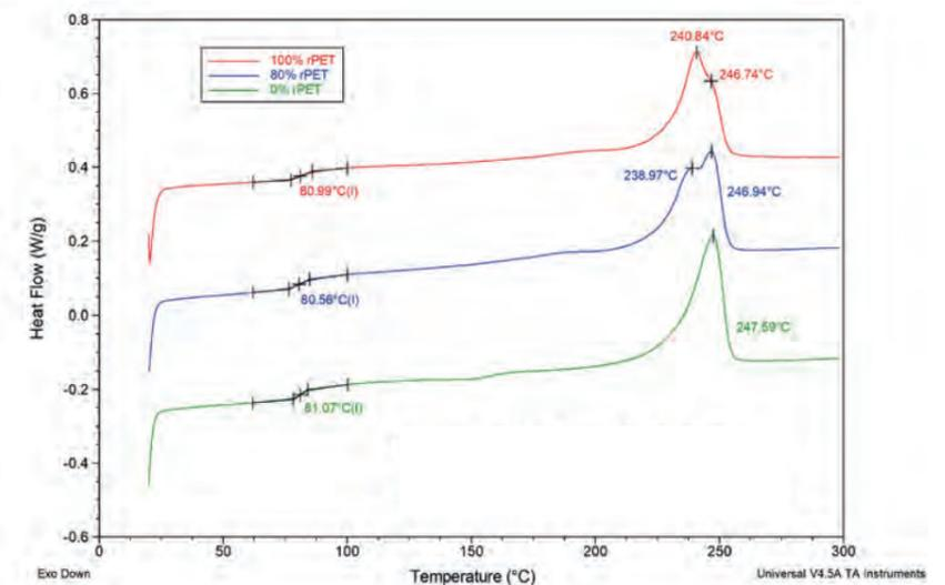
DSC Second heating: increasing rPET leads to changes in morphology, smaller crystals
