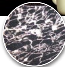
Area with stripes - particles with high content of pigment
