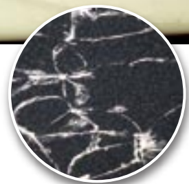
Area without stripes - particles with normal content of pigment
